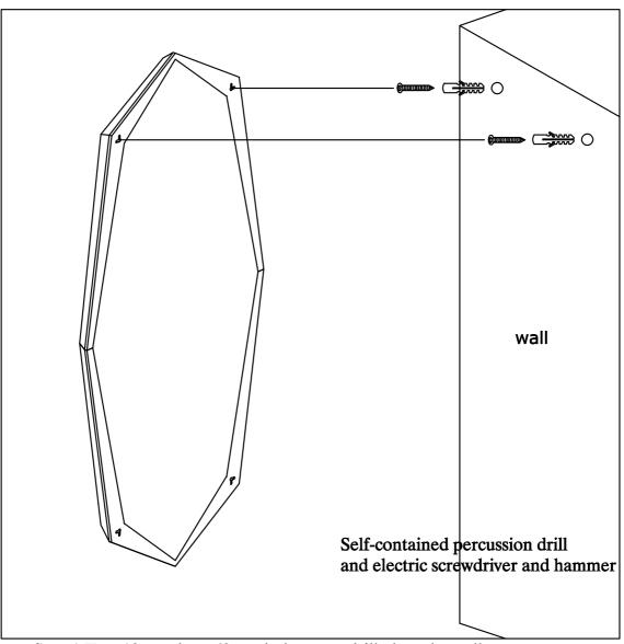
Step 1:Two 10mm deep 60mm holes were drilled on the wall with a percussion drill, and the expansion tube was punched into the wall with a hammer. Then the self-tapping screw was screwed into the expansion tube screw head with an electric screw to expose the wall for about 4mm. Finally, the mirror was hung on the wall by two people.
